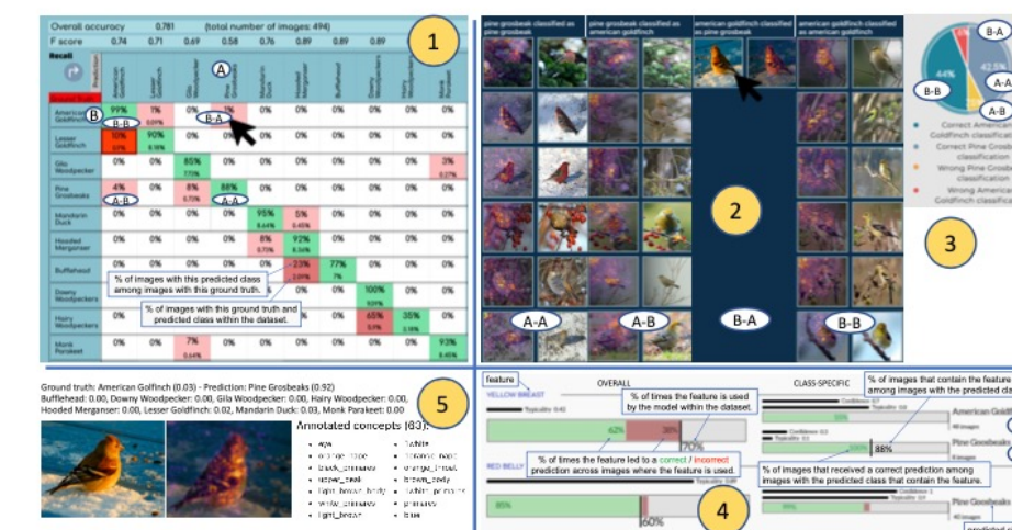
Fig. 2. Confusion matrix interactions. Our probe allows for different interactions with the explanations. For instance, when one clicks on a cell of the confusion matrix (1) corresponding to the predicted class A and ground truth class B, she is directed towards the corresponding local (2) (images corresponding to the cells A-A, A-B, B-A, B-B of the matrix) and global (3) explanations, as well as more performance indications (3). Clicking on a local, visual explanation displays further local, textual explanations (5).
